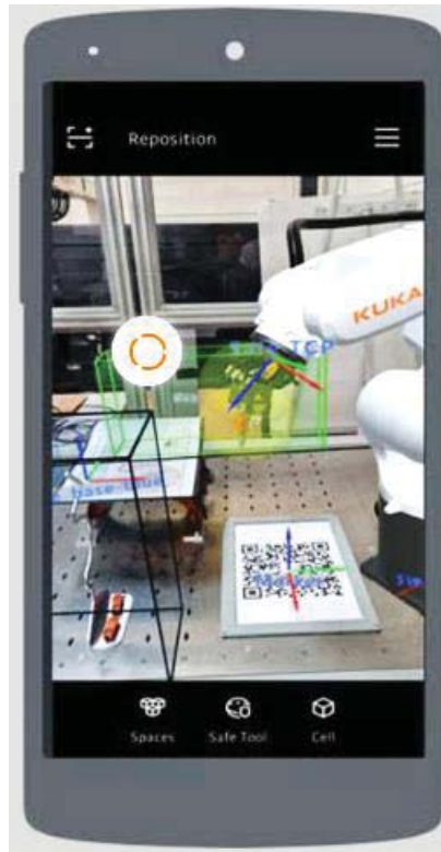
Figure 7. Robot programming using augmented reality
