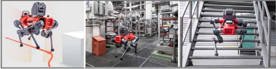
Figure 19. Autonomous mobile robot ANYmal from the ANYbotics Company for industrial plant inspections [52]
