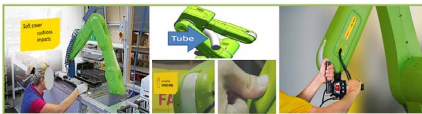
Figure 8. FANUC collaborative robot equipped with DCS (Dual Check Safety)safety system for tracking position and speed [37-39]
