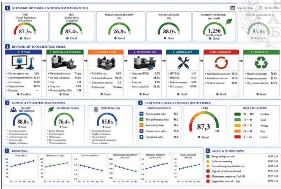
Figure 10. Integrated KPI dashboard for a plastic injection molding tool
