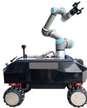
Figure 11. Autonomous mobile robot and collaborative robot equipped with multiple sensors.
