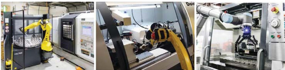
Figure 6. Collaborative robots performing CNC machine tending in manufacturing processes
