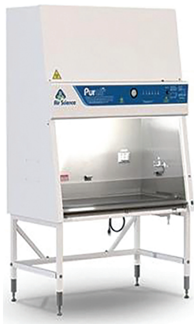
Slika 7. Biosigurnosni kabinet klase II (Izvor: Purair BIO Biological Safety Cabinets. NED Directory. https://directory.newequipment.com/classified/purair-bio-biological-safety-cabinets-252011.html (datum posljednjeg pristupa: 18. 1. 2024))
