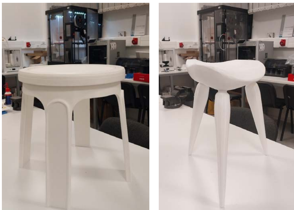
Figure 5. AI generated stool chairs after additive manufacturing
