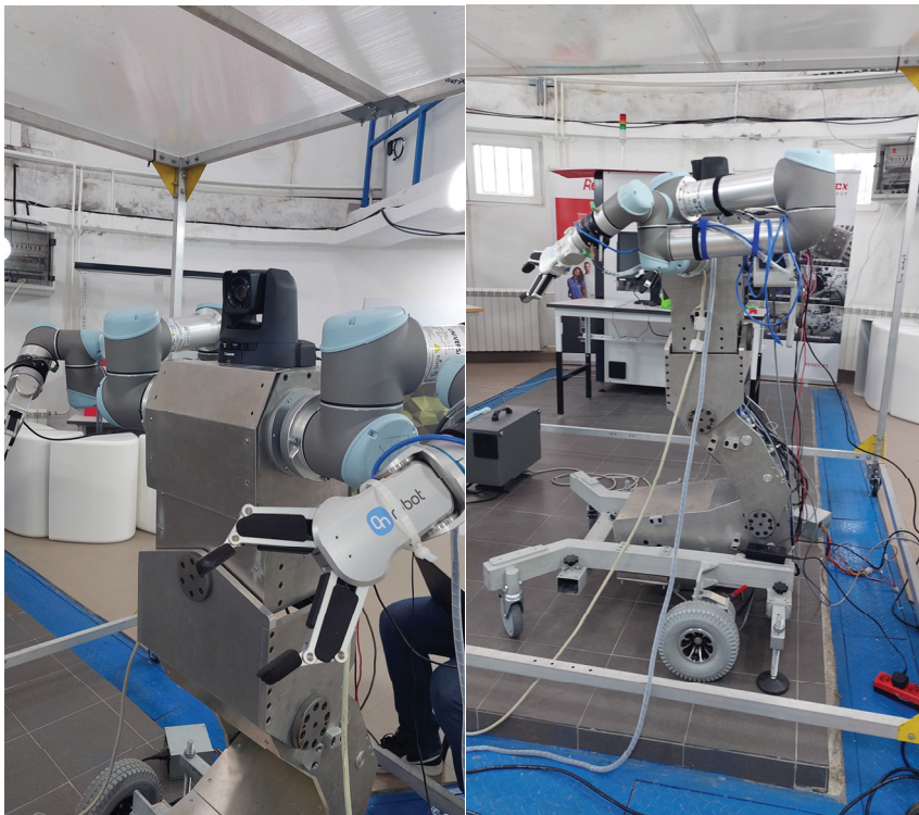
Figure 2. Laboratory prototype of the 21 DOFs bi-manual collaborative industrial humanoid developed in Mihajlo Pupin Institute – Belgrade [9]
