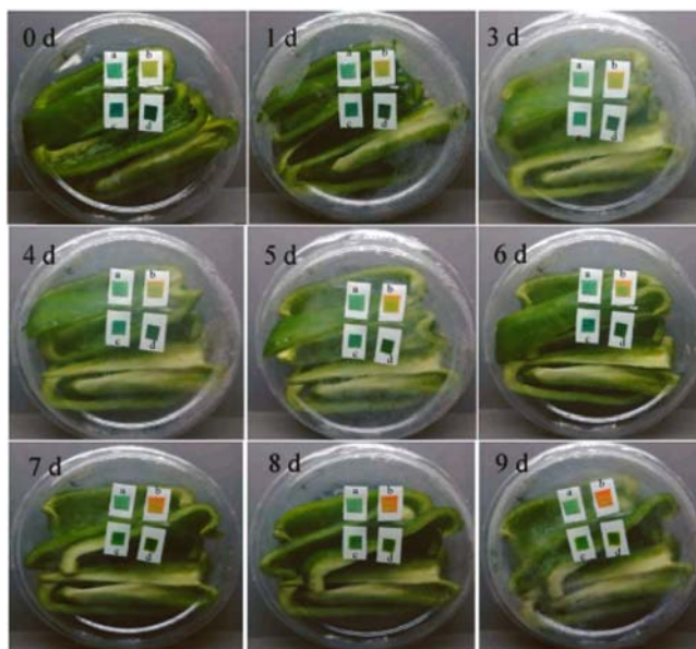
Figure 7. Freshness indicator application in food packaging
