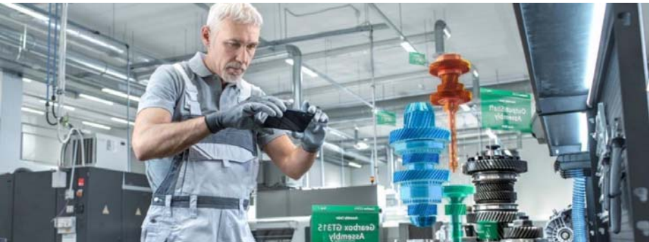
Figure 4. Interactive assembly instructions that recognize the components
