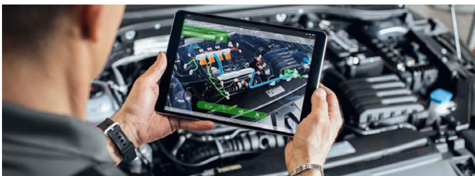
Figure 5. AR application for parts identification
