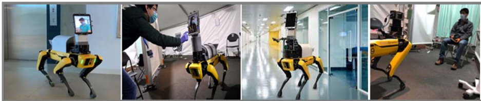
Figure 17. Implementation of Boston Dynamic Spot agile robot that assist in the treatment of patients suffering from the COVID-19 virus [50-51]
