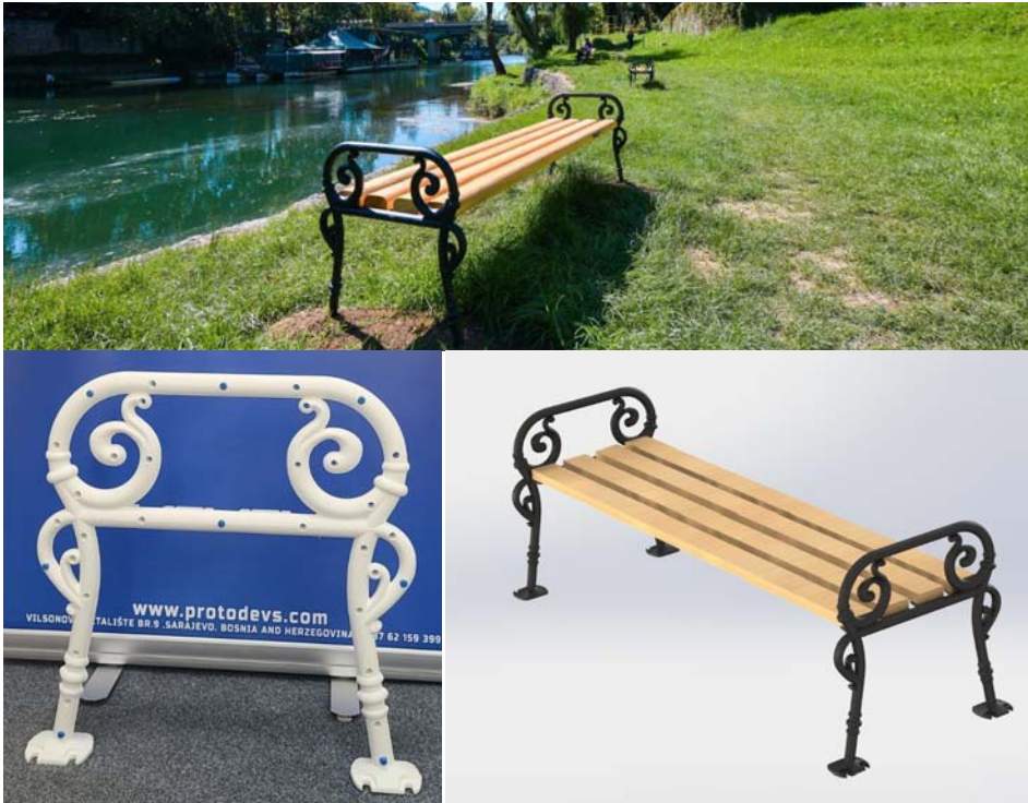
Figure 6. Park bench after 3D scanning, 3D printing and sand casting
