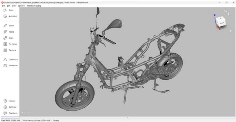
Figure 7. 3D scanned bike frame
