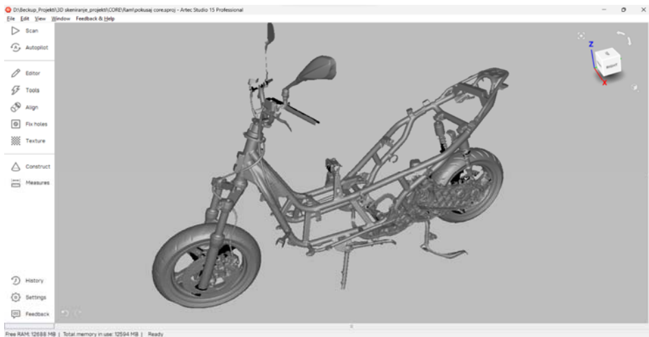
Figure 7. 3D scanned bike frame
